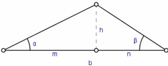
$$\left. \begin{array}{l} \tan \alpha = \frac{h}{m} \\ \tan \beta = \frac{h}{b-m} \end{array} \right\} \rightarrow \left. \begin{array}{l} m = \frac{h}{\tan \alpha} \\ \tan \beta \cdot \left( b - \frac{h}{\tan \alpha} \right) = h \end{array} \right\}$$
